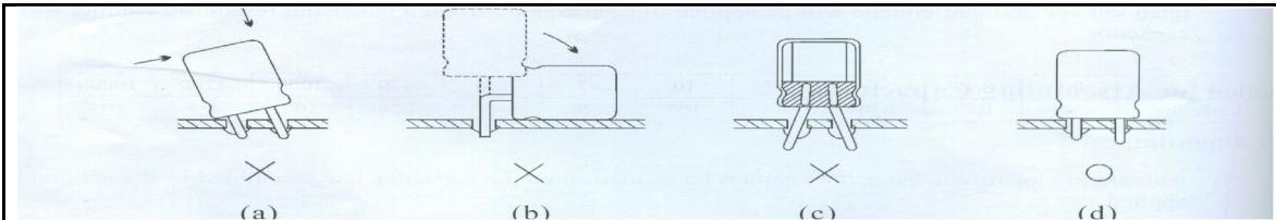
9、The aluminum case is not insulated from the cathode. Do not locate any copper or any via hole under the aluminum capacitors, on the PC board. Also, the dummy terminal is not insulated from the cathode. The dummy terminal must not be connected electrically to the anode .Other wise, both cases may cause a short circuit.
